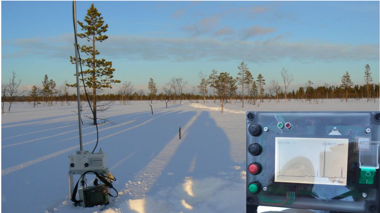
SnowMicroPen (SMP) – tool used to study snow layering without digging a snow pit. Device records the penetration resistance continuously. Peaks on controller panel indicates the hard (ice) layers within the snow cover.
