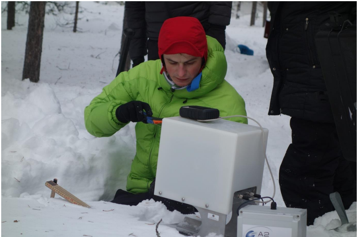
Bartek Luks during snow Specific Surface Area (SSA) measurements with IceCube. The operation of IceCube is based on the measurement of the hemispherical infrared reflectance of snow at 1310 nm (Photo by Martin Schneebeili)
