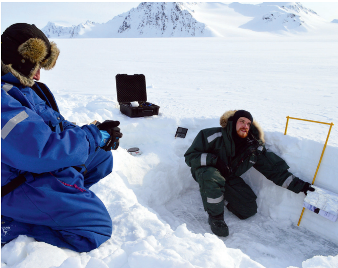
>> Measuring the thermal properties of snow cover using a thermal camera on the Werenskiöld Glacier in April 2016
