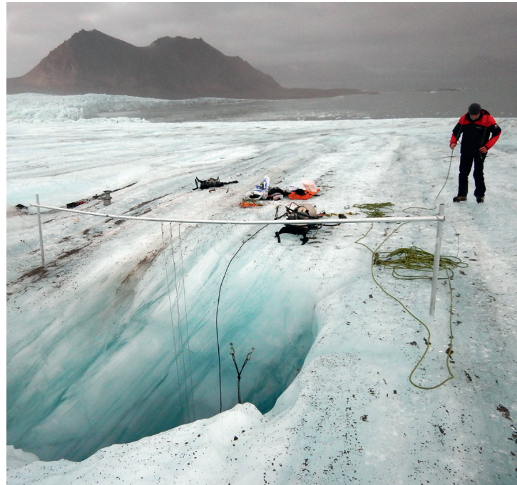
>> Metallic structure allowing to fix the cable on the glacier surface on which the sensors are attached on inside the glacier mill
