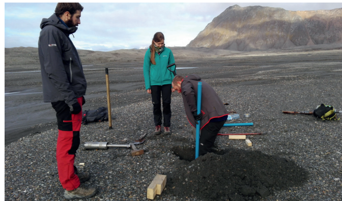
>> Installation of piezometers included in the hydrological monitoring network on the foreground of the Werenskiöld Glacier
